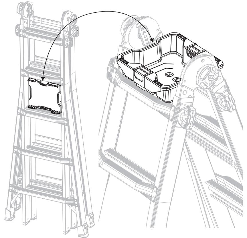
**WARNING:** Ensure bucket is securely attached onto the rungs before use.
